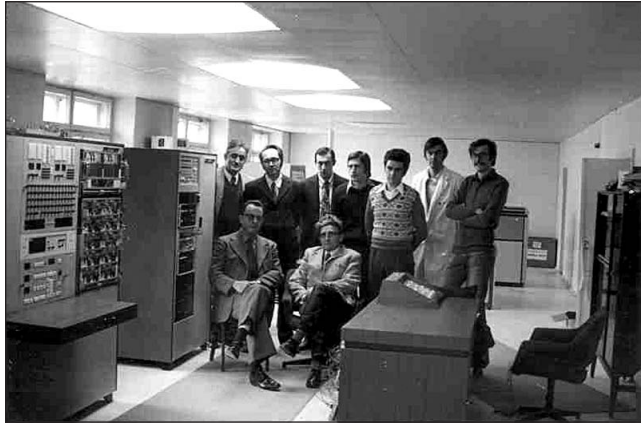
Figure 5. Image of a hybrid computer, model HCS-100, produced in Yugoslavia and put into operation at the Institute of Katalis Novosibirski branch of Academy of Sciences U.S.S.R. in 1975. This photo shows, from left, the analog part and box with A/D and D/A converters and desk with control console. The joint Soviet-Yugoslavian starting team is shown. Principal investigator Prof. B. Kogan and the vice-director of the Pupin Institute are seated from right to left. (From Boris Kogan's photo archive.)
